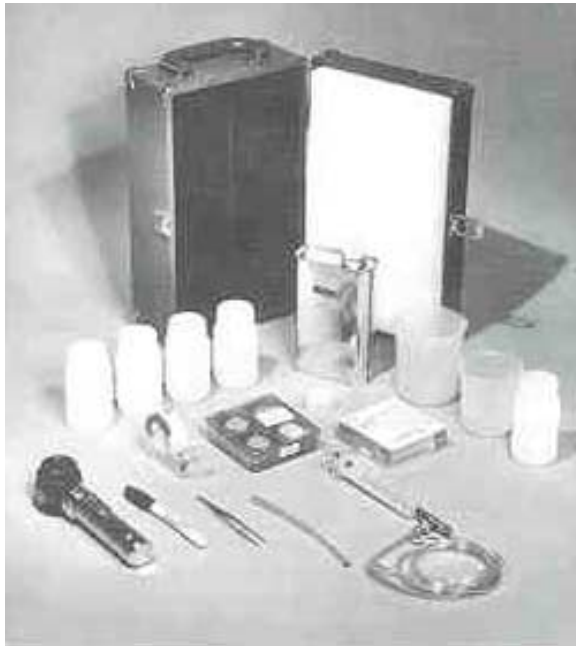
Figure 1. OILGEAR FLUID CONDITION KIT contents (55173).
