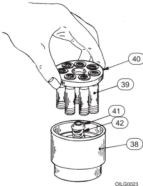
Figure 9. Rotating Group Disassembly
