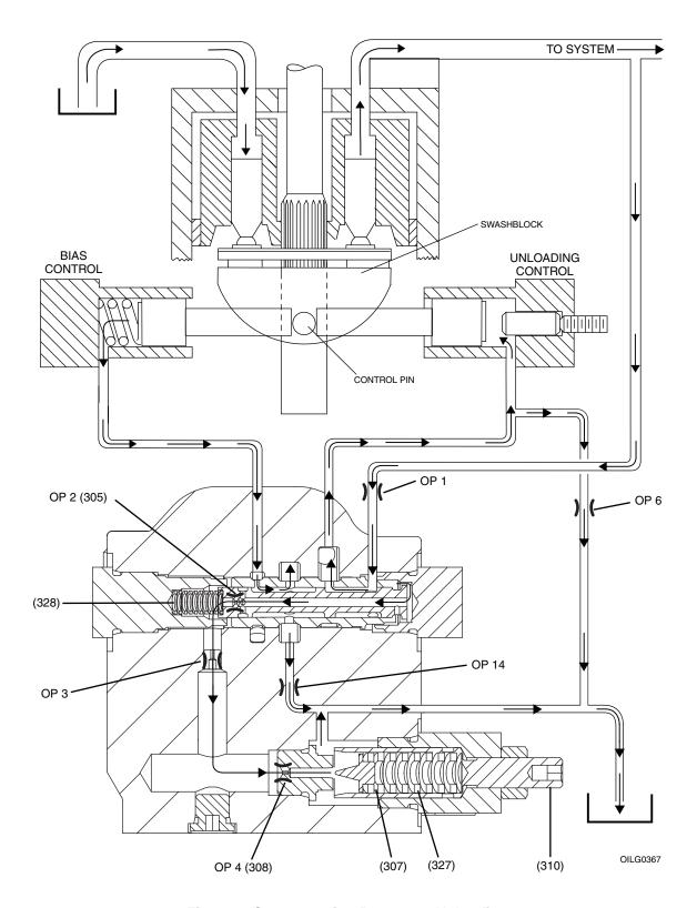
Figure 5. Compensating Pressure - Unloading
