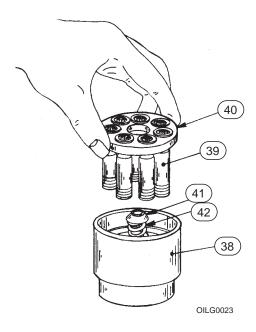
Figure 9. Rotating Group Disassembly
